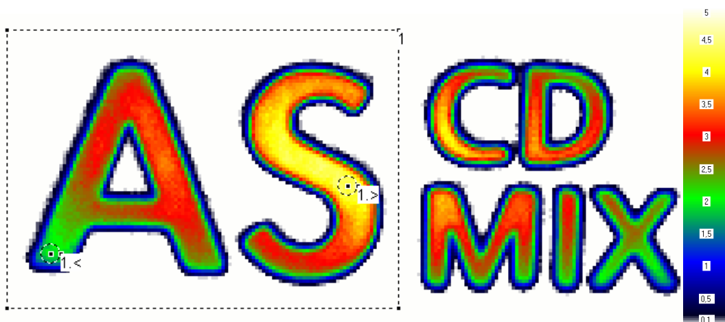
Diagram 1: Pseudocolor representation of the luminances of a symbol (palette on the right) The positions of the minimum (1.<) and the maximum (1.>) are defined by the circles drawn in the image.
