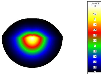
**Figure 1.** Luminance distribution weighted by Position Index (10 cd/m<sup>2</sup> of uniform luminance in equisolid pixel image).
