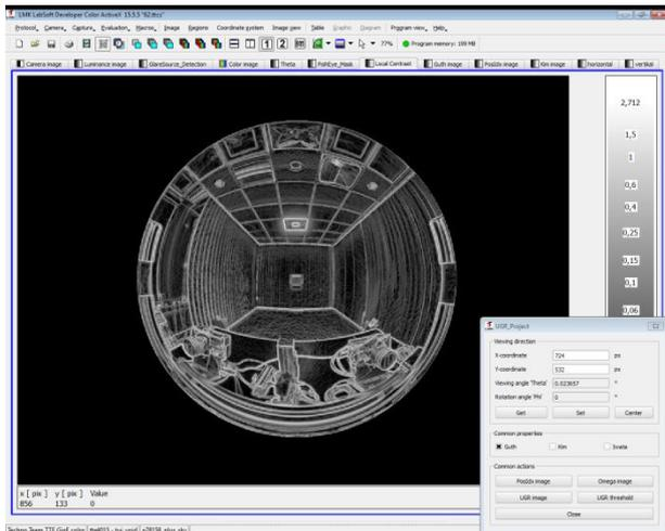
Figure 3 – Local contrast before binarization with a threshold of  $C_{loc.th} = 0.25$
