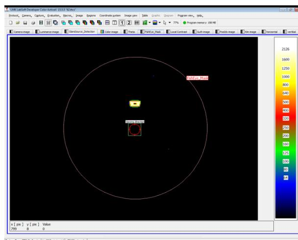
Figure 8 – Luminance image only containing detected glare sources
