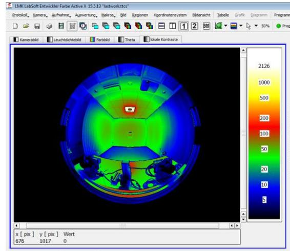
Figure 4 – Local contrast threshold ( $C_{loc.th} = 0.25$ ) filtered luminance image
