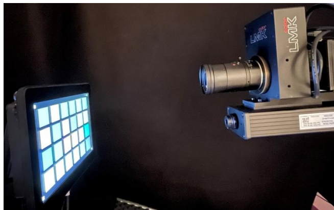
Figure 15: LMK Position with spectrometer option: After the camera alignment, LMK Position can be switched to spectrometer mode to place the JETI specbos optical axis and entrance pupil to that of the LMK
