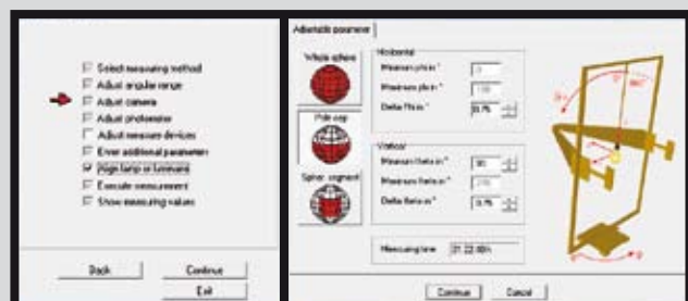
Guided measurement setup steps / setup of angular range and resolution
