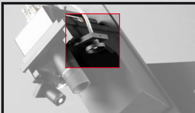
Spectrometer detector head mounted on RIGGO 801 LED
