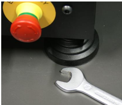
Figure 17: open-end wrench for turning the mounting feet
