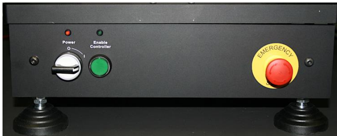
Figure 14: Emergency-stop switch at front panel
