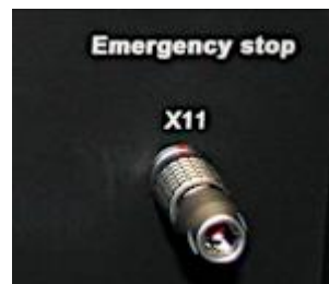
Figure 15: Emergency-stop circuit connector at the back panel
